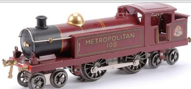
EMR/1 108 Metropolitan maroon gloss or matt Issued in 1996. This model was based on the No.2 Tank Engine in the pre-war Hornby Series, which went out of production in 1929. The original models were available only with a clockwork mechanism but the E/1 locomotives by ACE Trains have 20v electric mechanisms with remote control in AC/DC.
